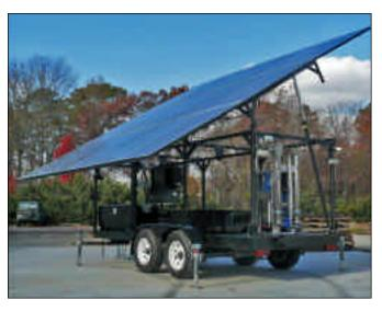
Mobile solar powered units can be system integrated, engineered and designed to produce safe drinking water dependably and economically from a wide range of problem input sources. The systems are well suited for various applications in areas with no power and poor water quality.
